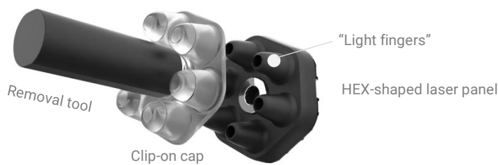
Graphic 13: Replacement of a disposable cap with magnetic removal tool
